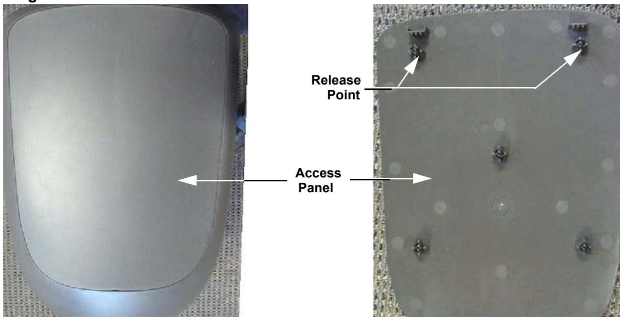
4. Remove the two screws in the rear of the cover assembly and the mounting screw shown in Diagram 7.2. Carefully pry the two snaps, shown in Diagram 7.2, toward the rear and remove the top cover.
