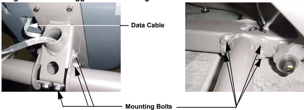
5. Loosen but do not remove the two clamp bolts at the handlebar pivot point. See Diagram 7.25.
