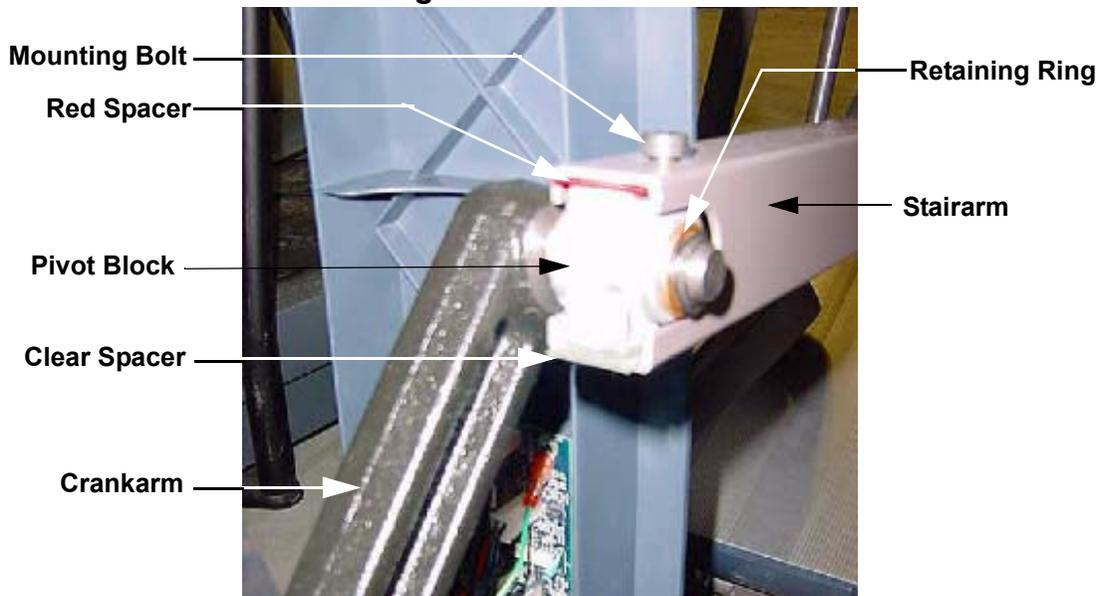
7. Slide the stairarm pivot block onto the crankarm pin and replace the wave washer, flat washer and retaining ring removed in step 6.
