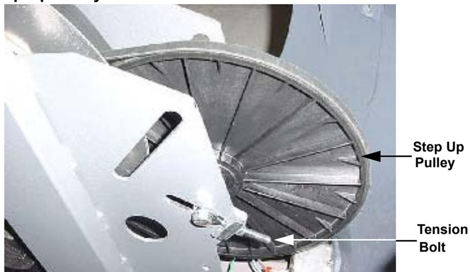
9. Remove the input pulley belt and place the replacement input pulley belt in its place on the step up pulley assembly.
