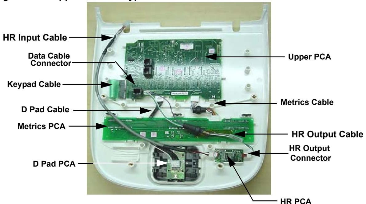
6. Set the display back in its mounting position and reconnect the data cable. Set the on/off switch in the “on” position.
