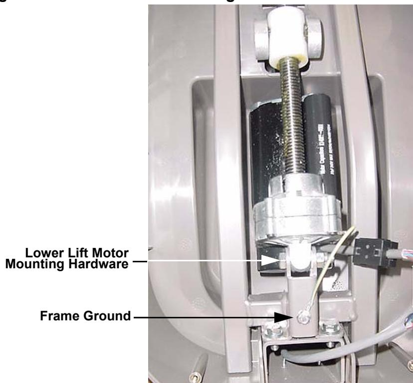
6. Disconnect the lift motor cable connector.
