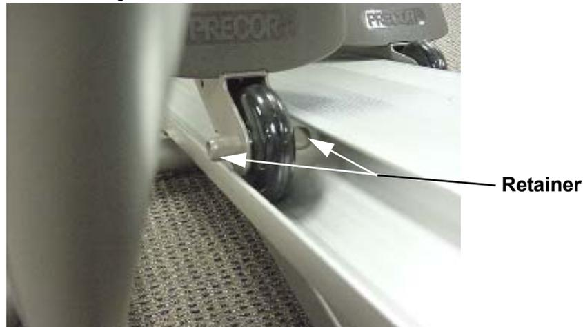
6. Remove the screws that fasten the two retainers to the stairarm. Remove the wheel and discard.
