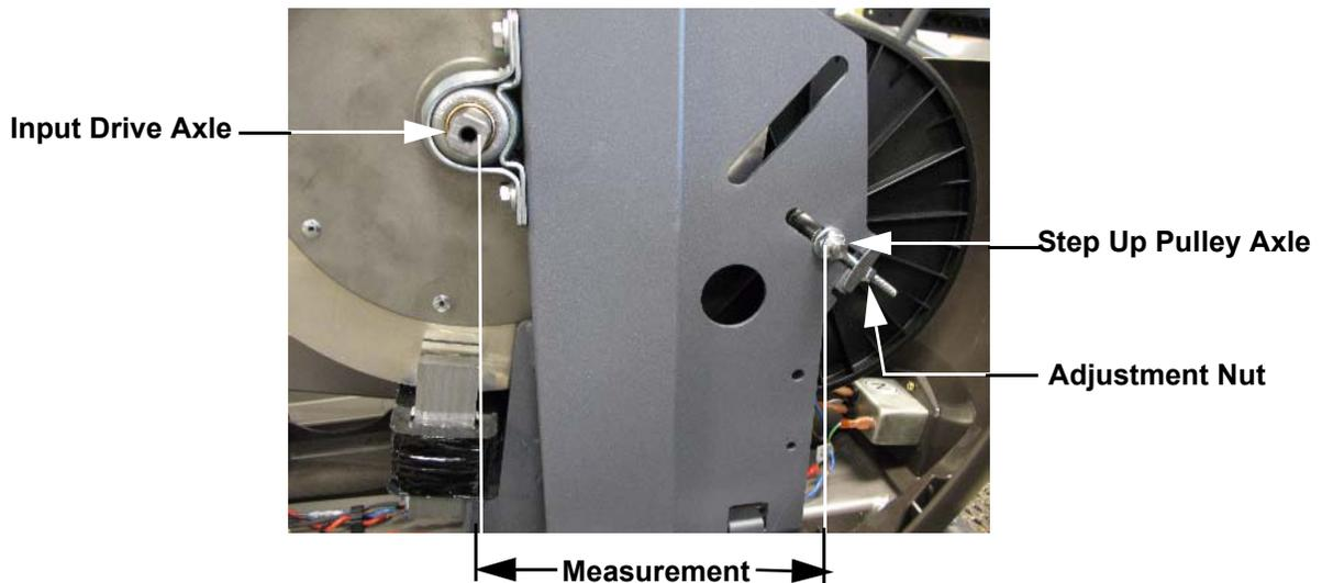
10. If the difference between the two measurements is greater than 1/16 inch, continue with step 11. If the difference is less than 1/16 inch, skip to “eddy current magnet adjustment”.
