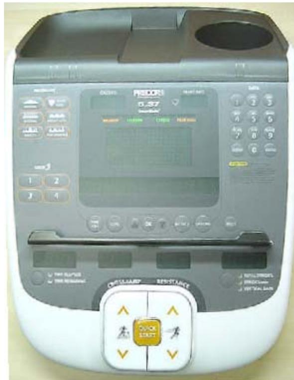
3. The test name **HARDWARE VALIDATION** will be displayed. Press the **OK** key to proceed to the display test.
