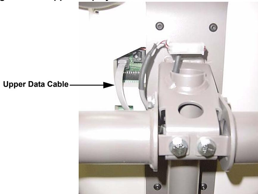
12. If the upper data cable corrects the problem, replace the cable. If the upper data cable does not correct the problem, re-connect the original upper data cable to the mid-point connector and the upper PCA and continue with step 12.
