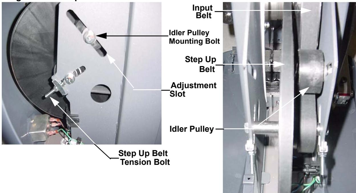
5. Tighten the idler pulley mounting bolt to the settings marked in step 3. Torque the idler pulley mounting bolt to 120 inch pounds (10 foot pounds).
