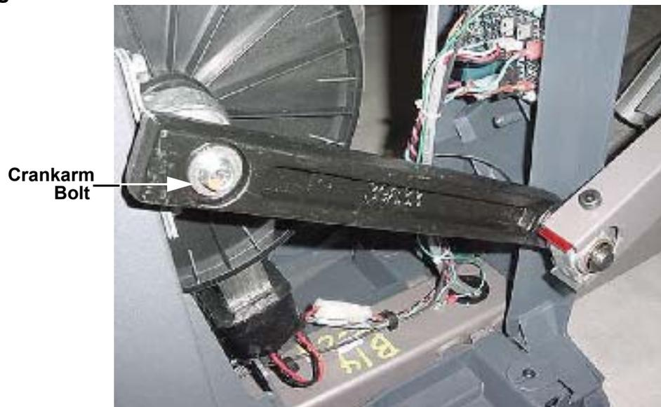
6. Clean the crankarm mounting bolt threads and the input pulley shaft threads with an alcohol swab. Allow them to dry and apply blue loctite to the crankarm mounting bolt threads.
