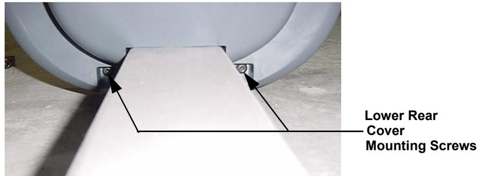
7. Raise the incline to its highest position. Remove the two screws from the rear of the lower portion of the rear cover. See Diagram 7.22.
