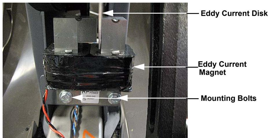
16. If the eddy current disk is not centered, loosen the two eddy current magnet mounting bolts and move the magnet to center the eddy current disk.
