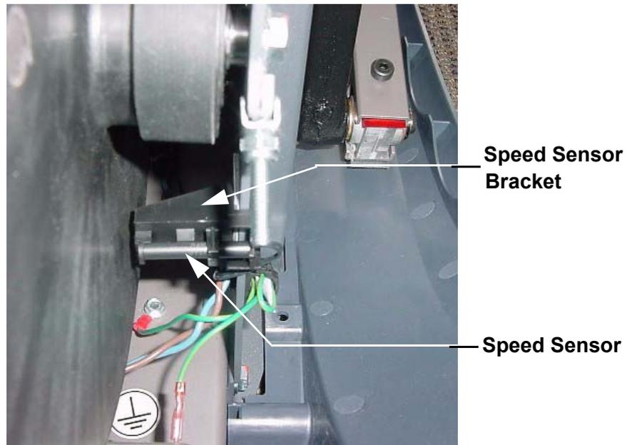
6. Snap the replacement speed sensor into the speed sensor bracket. See Diagram 7.9.
