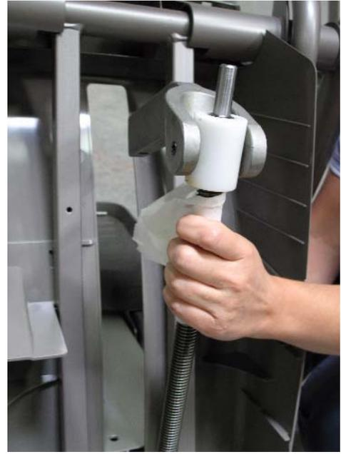
9. Note the orientation of the incline yoke, the replacement yoke must be installed in the same orientation. If the replacement yoke is installed upside down the incline will go too low and damage the cover. See Diagram 7.31.
