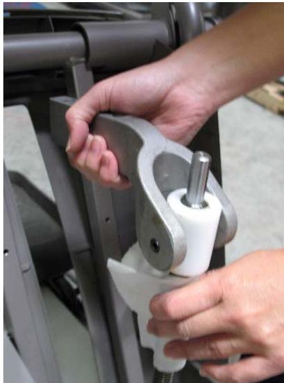
11. Taking care to not allow the incline motor's drive screw rotate, correctly orient the replacement incline yoke and thread it onto the incline motor's drive screw until it is in the same position as noted in step 5. If the incline motor's drive screw rotates, the incline motor will need to be calibrated per Procedure 5.3.
