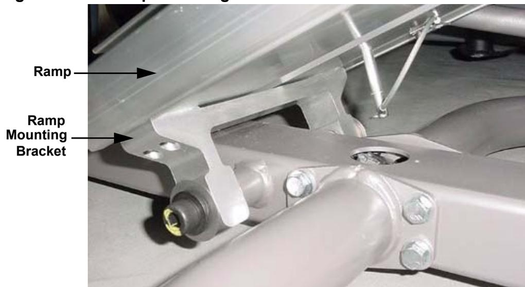
5. Remove the two large bolts that fasten the ramp mounting bracket to the frame.
