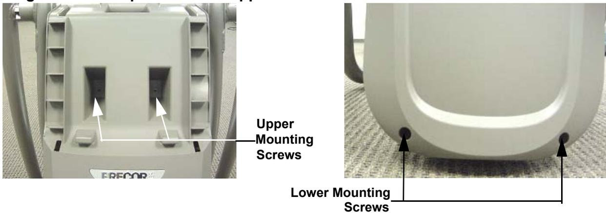
5. The lower rear cover must be removed before the upper rear cover. Plug the power cord in the A.C. outlet and set the on/off switch in the “on” position. Lower the incline to its lowest position.
