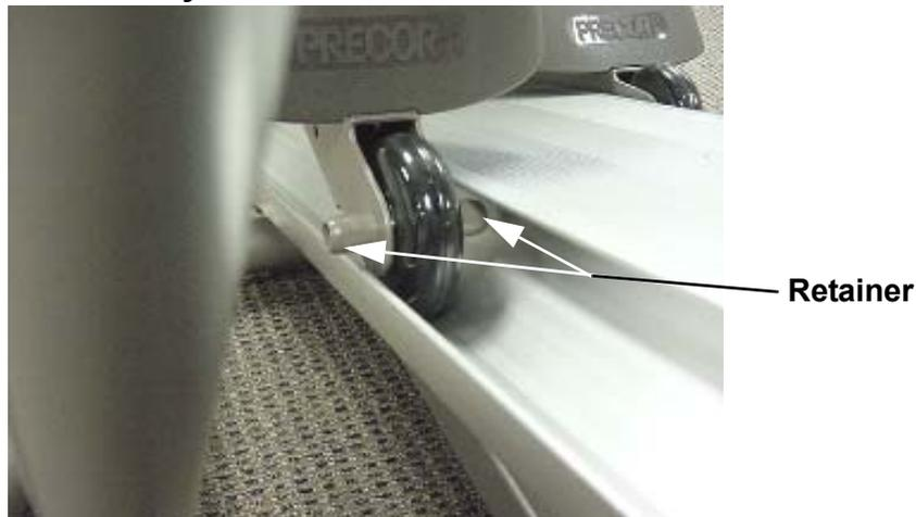
6. Remove the screws that fasten the two retainers to the stairarm. Remove the wheel and discard.
