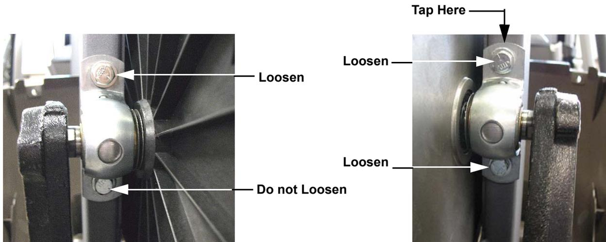
6. Using a rubber mallet, gently tap the top of the pillow block with two loosened bolts (the right hand pillow block in Diagram 5.7) until the two measurements in Diagram 5.6 are within 1/16 inch.
