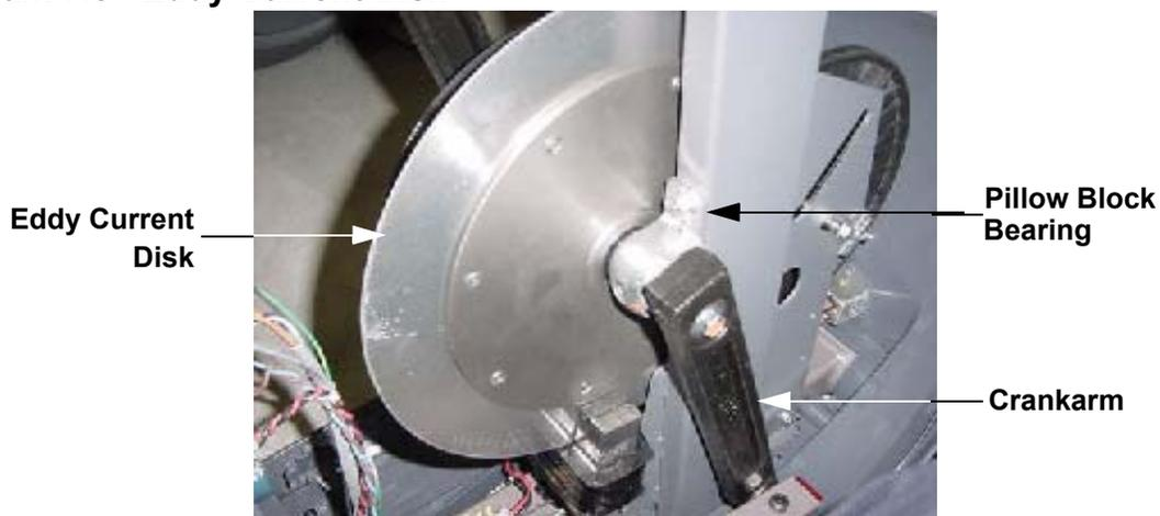
7. Slide the step up and input belts onto the replacement input drive assembly as you set the input drive assembly in it's mounting position in the EFX.
