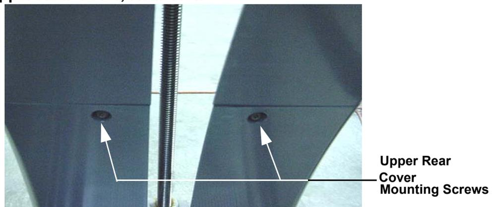
8. Lower the incline to its lowest position, set the upper rear cover in its mounting position and fasten it with the two screws removed in step 7.
