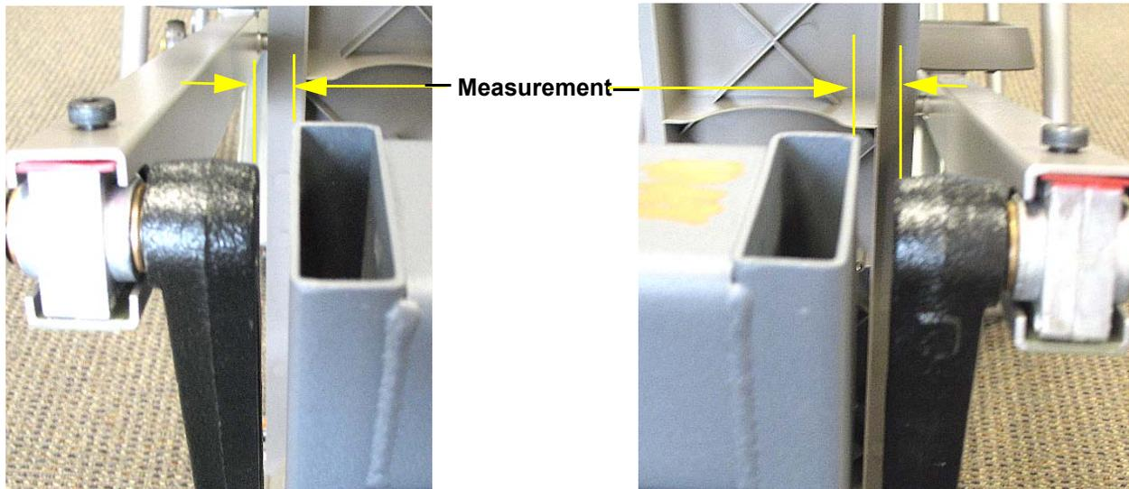
5. On the side with the larger measurement, loosen the upper pillow block mounting bolt only, do not loosen the lower pillow block mounting bolt. On the side with the smaller measurement, loosen both pillow block mounting bolts. See Diagram 5.7. For purposes of illustration we will assume that the left measurement was larger than the right side measurement in Diagram 5.6.
