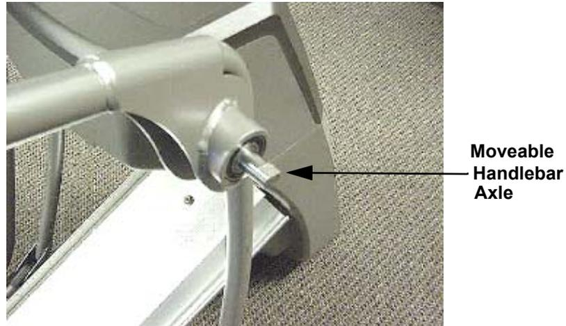
6. Set the replacement moveable handlebar in its mounting position. Carefully start hand threading the moveable handlebar to avoid cross threading and then tighten..
